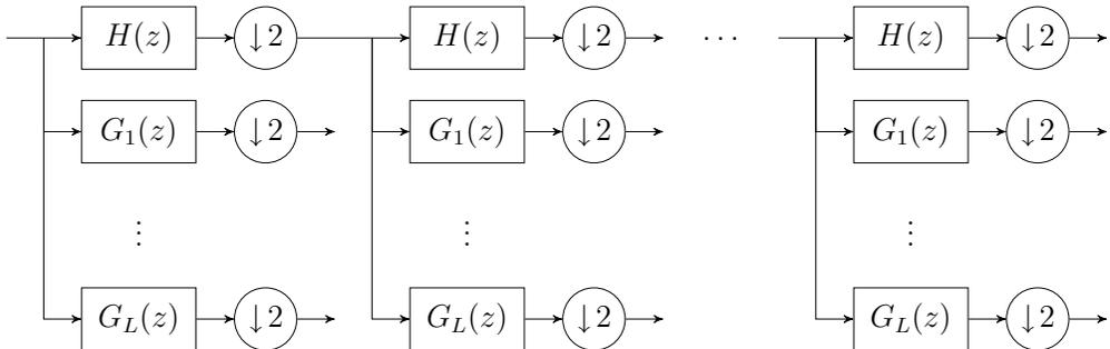
Fig. 6. An overcomplete FB obtained by iterating the lowpass branch of an overcomplete  $L + 1$  channel FB.
