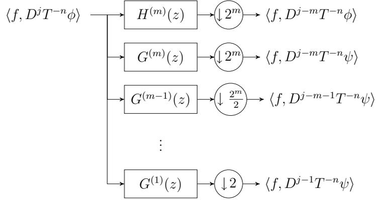
Fig. 4. The iterated FB in Figure 3 with  $m$  stages is equivalent to the  $m + 1$  channel FB above.
