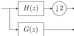
Fig. 2. This filter bank can not generate a tight frame for  $l_2(\mathbb{Z})$  if FIR filters are used (also see [10] for a further discussion).
